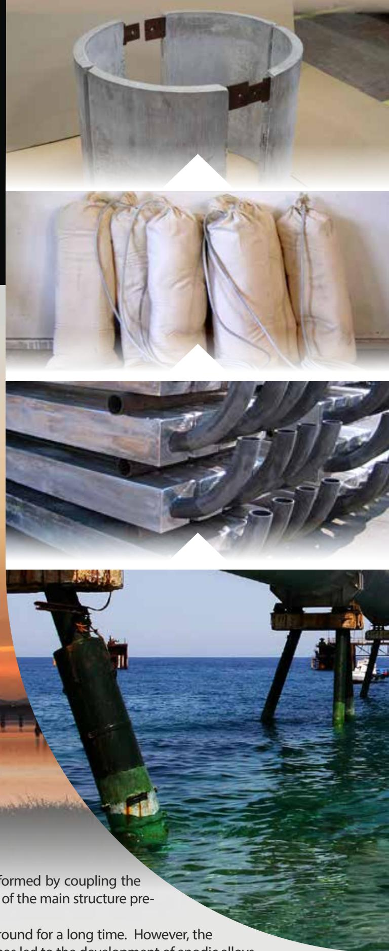
The cathodic protection of a metal structure can be performed by coupling the metal with a less noble material, that will corrode instead of the main structure preserving it over time (sacrificial anodes).
